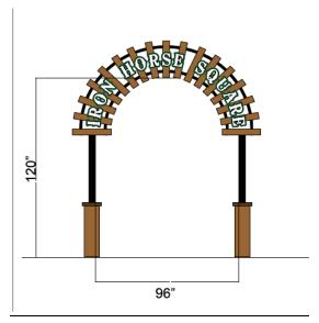
Sign will be a replica of crossties & rails with letters "IRON HORSE SQUARE". All will be metal except for the brick work at the base of the upright posts.
