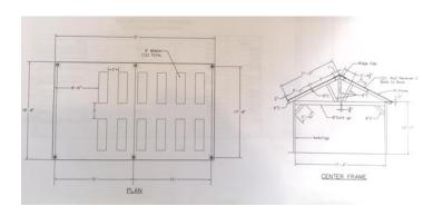
Covered open air pavilion with seating for 36. A 3' railing around perimeter with a gate which opens onto a loading dock for convenience of loading passengers onto train. (full set of architect drawings are available)
